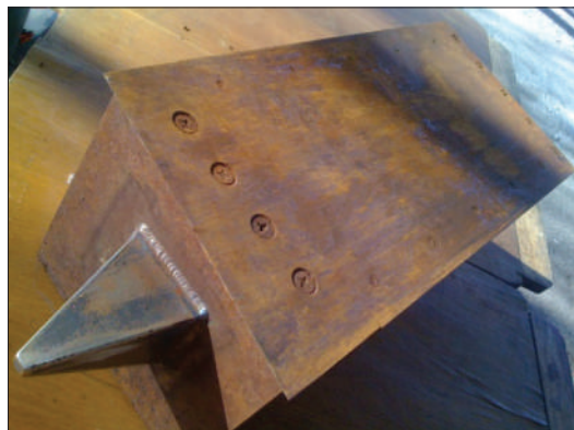
Fig. 5. Piston of Plunger System of Polymer Wastes Supply with Truncated Pyramid on the Front Plate (Variant 4, c)
