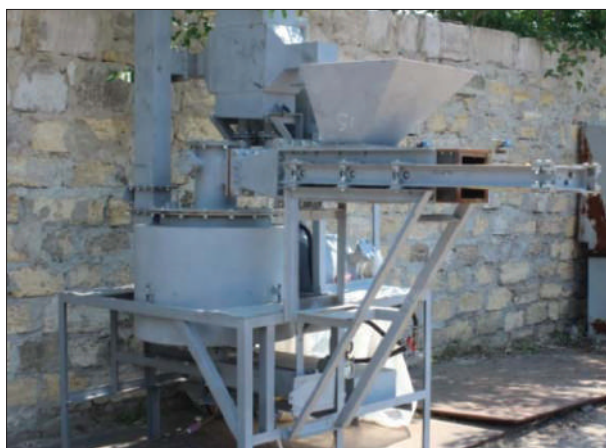
Fig. 1. The Ecopir-18 MCP Experimental Plant with Plunger System of Continuous Polymer Waste Supply into the Reactor
