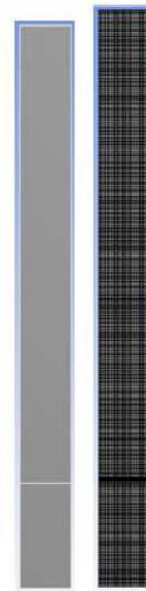
Fig. 9. 3D model of the rod and its division into finite elements
