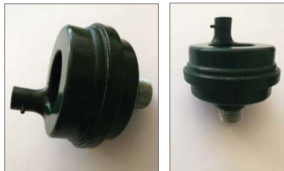
Fig. 7. Test sample of the oil separator with the productivity of G = 2 - 10 m^3/h
