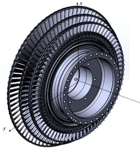
Fig. 1. Gas turbine rotor in the Cartesian right-handed coordinate system.
